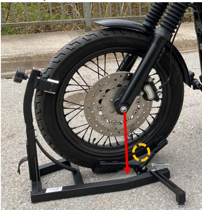
The axle center of the front tire (red line) must be slightly in front of the tilting axis (yellow) of the lower crab after pushing the motorcycle into the stand as shown in the image.
