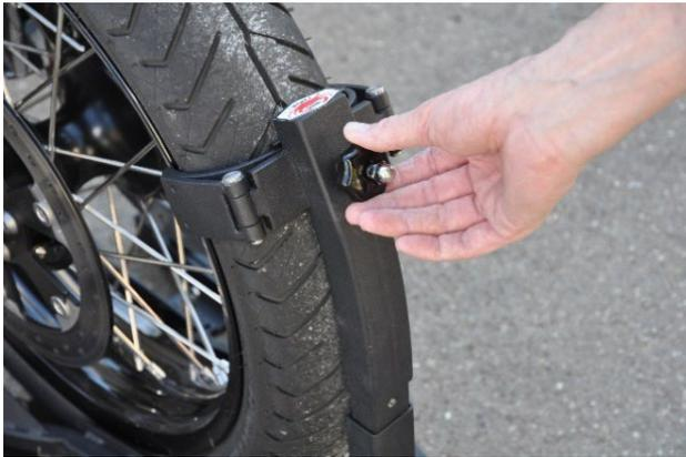
25. To prevent theft, the upper crab can be locked with a security lock (optional accessory). The knurled screw can then no longer be opened.
