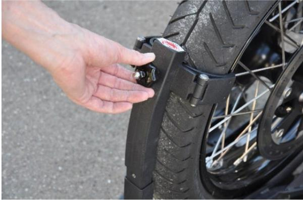
When the two-wheeler is moved out, the two crabs open automatically and release the tire.
