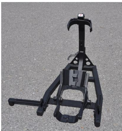
21. For small uneven surfaces, you can further increase stability by unscrewing the height-adjustable machine foot until Moto-Crab rests firmly on the ground.
