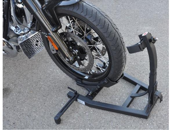
The lower crab closes around the tire when the tilt axis is overcome.
